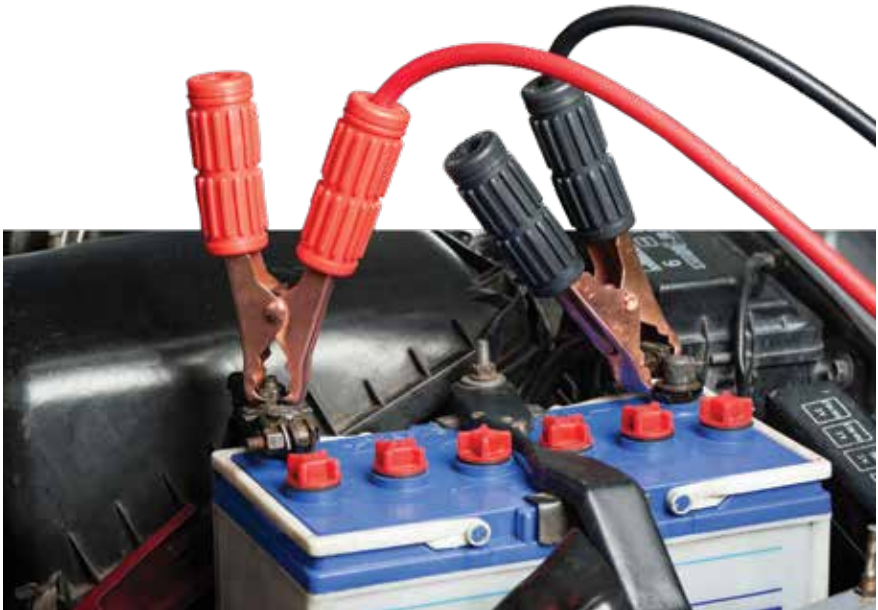
Correct jumper cable connections
