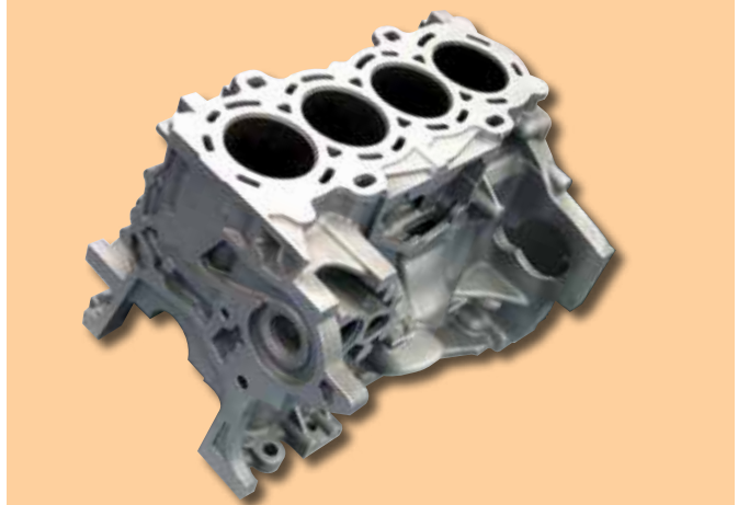
The inline-4 is the most common engine configuration.
